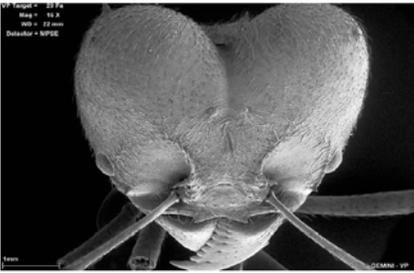
*Low magnification image at a long working distance. This image illustrates the excellent high signal level in VP mode at 20Pa without any shadowing on this highly topographic sample.*
